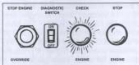
Typical Shutdown Override Switch and Engine Lights
